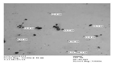
Fig. 2. Transmission Electron Microscopy (TEM) image of Ag-NPs with spherical shapes (sizes ranged from 8.55 to 20.3nm).
